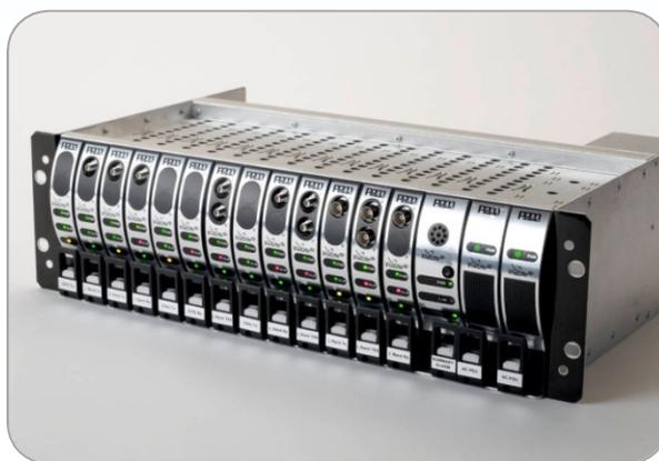
The **ViaLiteHD** wide dynamic range broadband fibre optic links have 0dB link gain. For installations where the number of cross site fibre connections is limited the complete ITU range of CWDM transmitter wavelengths is offered allowing up to 18 channels to be carried on one fibre. Optical connector options include FC/APC, E2000/APC, SC/APC and LC/APC.
