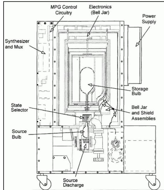
**FIGURE 2:** MHM-2020 Active Hydrogen Maser - Internal View
