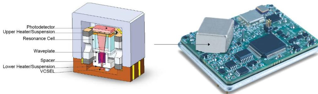
The center stack consists of a special-purpose VCSEL, the atomic vapor resonance cell, and the photodiode. The laser light, emerging from the VCSEL, diverges as it transits a cell spacer before passing through the resonance cell, and is detected on the photo detector. The center stack must be temperature-stabilized at a specific temperature, between 85 °C and 95 °C, which is precisely determined by the characteristics of the individual VCSEL device.
